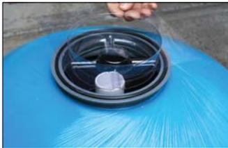
3. a. Fill the filter tank with water, until it is at least half full. This is done so that the weight of the sand media does not damage the underdrain at the bottom of the tank.
