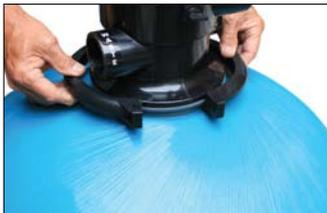
b. Remove the MP Valve from the tank top.
